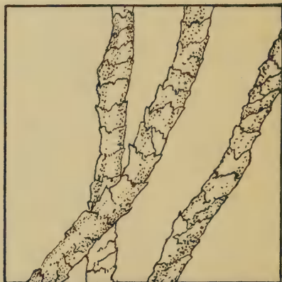
FIG. 191. — Notice the scale-like appearance of the wool fiber. Of what use are these scales?
